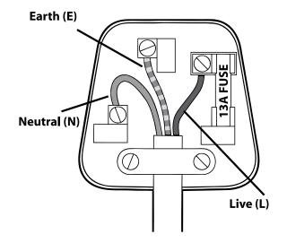
The wire which is coloured BLUE must be connected to the terminal which is marked with the letter "N" or coloured BLACK.
