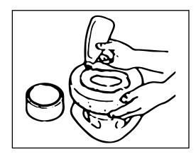
Spread the polishing paste evenly over the polishing pad. do not apply the polish directly to the polishing surface.
