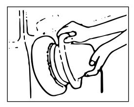
Work next on the smaller surfaces (doors, for example). allow the mains cable to hang from the appliance and hold the polishing machine as illustrated.
