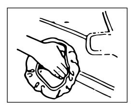
For less accessible areas (such as wing-mirrors, bumpers and door handles etc) remove the polishing cap from the pad and polish these areas by hand.
