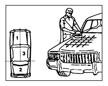
Place the extension lead over your shoulder and work first on the large flat surfaces such as the bonnet, boot lid and roof, keeping your movement as regular as possible.
