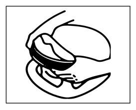
Now replace the textile polishing cap With the fine polishing cap and pull this over the polishing pad. Make sure it is completely clean. Remove the layer of polish in the same order as it was applied .important! Do not exert pressure on the polishing machine!
