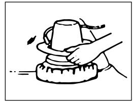
Switch the polishing machine on and off only when the polishing machine is resting on the polishing surface.
