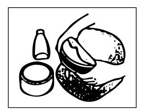
Pull the textile polishing cap over the polishing pad. Make sure the polishing cap Is completely clean.
